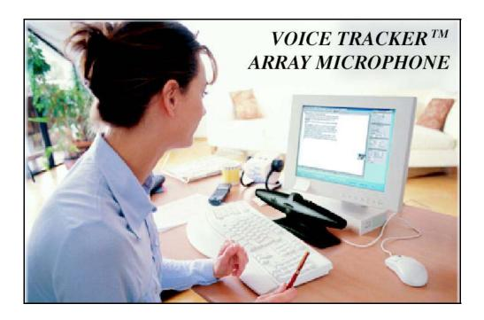
Unlike 1st generation array microphones which have a fixed "listen" direction, the Voice Tracker<sup>TM</sup> Array Microphone automatically locates and electronically steers toward the talker.
