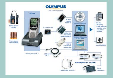
Data Transfer via Docking station The optional docking station is not just a DS-2300 cradle for your desk, it also allows connection via USB cable for fast up/download of voice files to the PC or Mac.
